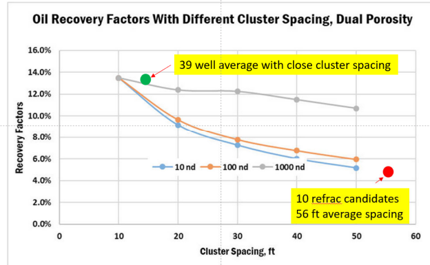
Fig. 10—Recovery efficiency based upon the dual-porosity model at the end of year 30.
